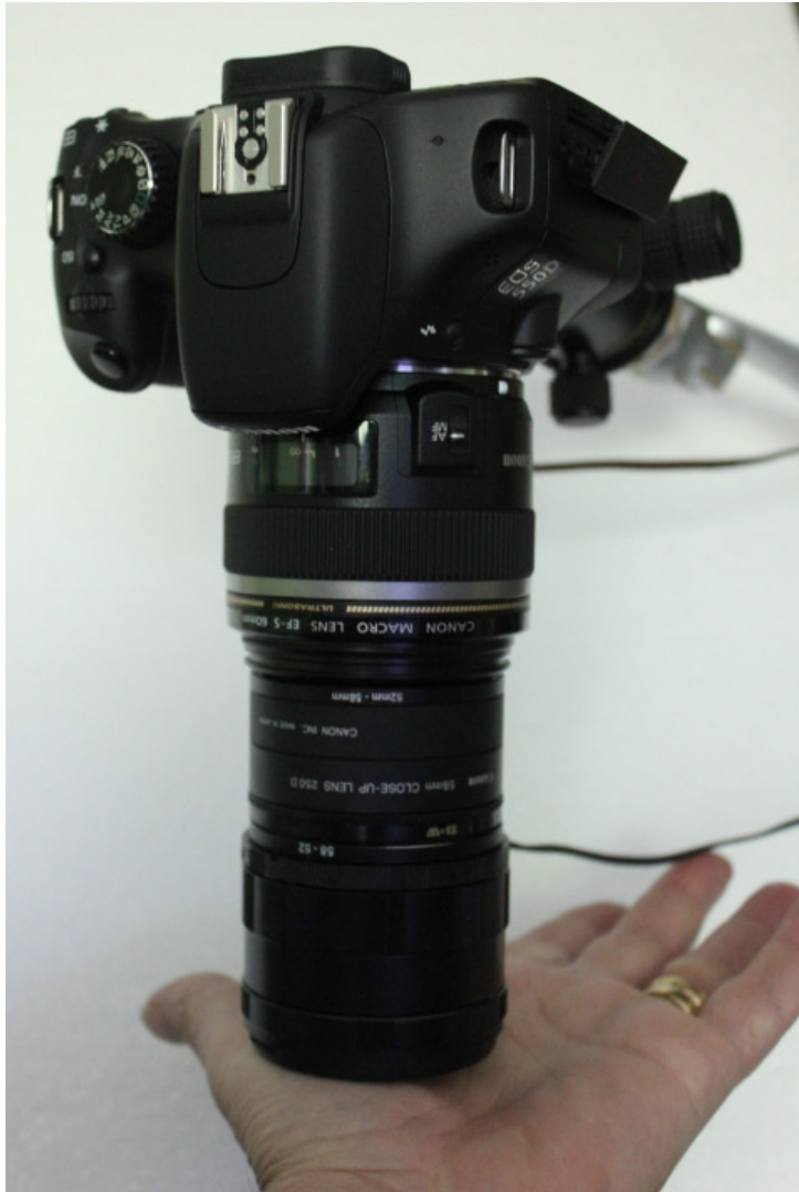
Fig 1. The TiVi camera equipped with the TiVi Camera Microscope adapter in measurement position over the palm of the hand.
